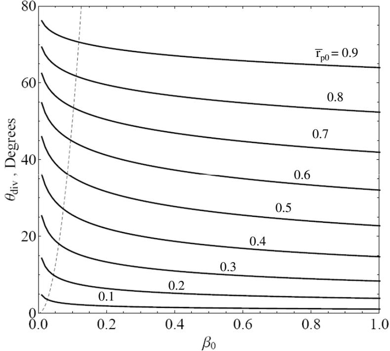
Figure 3. Divergence angle as a function of  $\beta_0$  for different values of  $\bar{r}_{p0}$  as obtained from Eq.(30). The dashed line qualitatively indicates a transition region between large divergence angle improvements and marginal improvements for increasing  $\beta_0$ .
