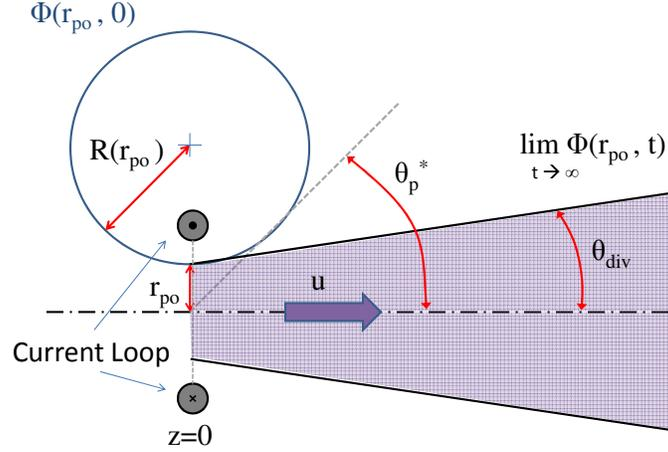
**Figure 2.** Diagram describing the definition of the initial magnetic field orientation at the plume edge,  $\theta_p^*$ . Also shown is the geometry of the estimated flux line used to express  $\theta_p^*$  in terms of  $\bar{r}_{p0}$ .
