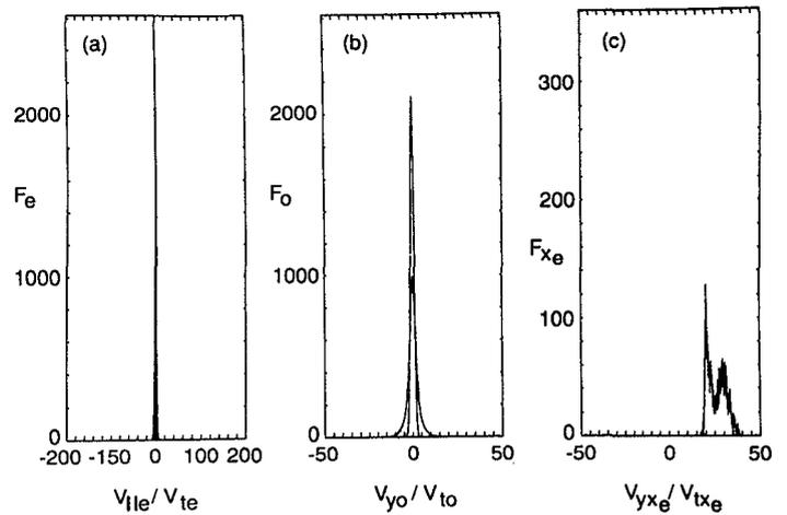
FIG. 5. The velocity distributions for the electrons [panel (a)], oxygen ions [panel (b)], and xenon ions [panel (c)] at  $t=0.4$  ms. It is shown that acceleration of the electrons along and oxygen ions across the magnetic field began to take place as a result of the plasma instability near the oxygen lower hybrid waves. The delta-function-like distributions in panels (a) and (b) correspond to the initial electron and oxygen ion distributions at the ionospheric temperature.
