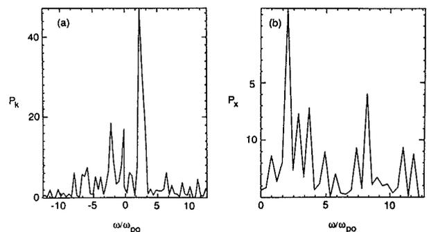
FIG. 6. Power spectra of the charge density for a Fourier mode  $(m,n)=(4,3)$ , (a), and at a location near the neutral gas in the  $(x,y)$  plane, (b). Note for both cases, a peak near  $2.0\omega_{po}$  is clearly seen, which corresponds to the oxygen lower hybrid wave.
