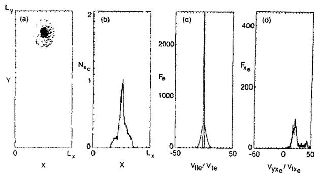
FIG. 7. Results of the simulation at  $t=0.7$  ms for the xenon ion cloud produced by the electron impact in the  $(x,y)$  space [panel (a)], its average density in  $x$  [panel (b)], the electron velocity distribution [panel (c)], and the xenon ion velocity distribution [panel (d)].
