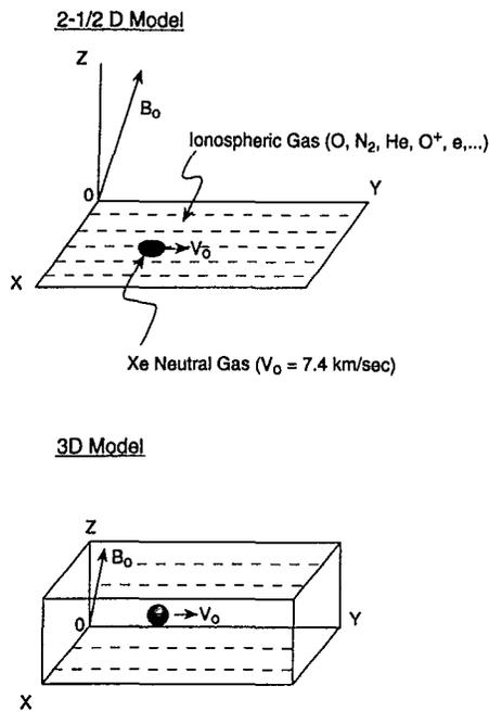
FIG. 1. Sketch of the numerical simulation models developed to study neutral gas release experiments into the ionosphere. A two-and-one-half-dimensional model (top) has two spatial coordinates,  $x$  and  $y$ , and three velocity components. Extension to a three-dimensional model (bottom) is straightforward.
