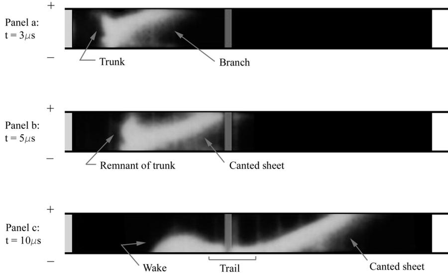
Figure 1: Photograph of the discharge at  $t = 3, 5,$  and  $10 \mu s$ . (The vertical grey object at the left of the accelerator is an insulator backplate, and at the center is a post that blocked the camera.) From reference [12].
