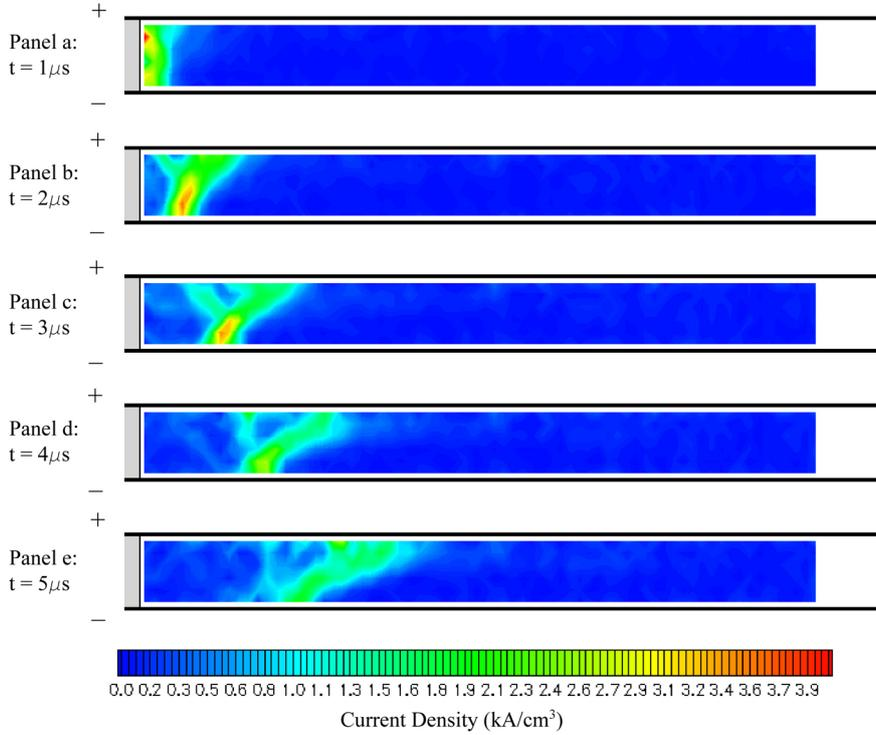
Figure 5: Current density contours at  $t = 1 - 5\mu s$ .
