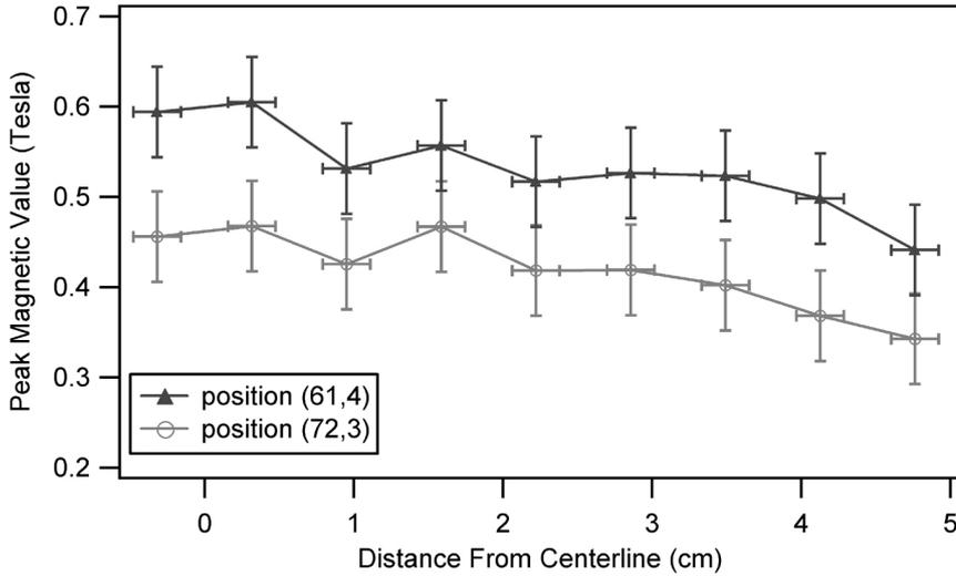
Figure 6: Peak magnetic field values vs. distance from the center in the  $z$  dimension for two different  $(x,y)$  positions. The error in the magnetic field measurement is taken as the largest standard deviation from repeatability tests, as discussed in section 3.
