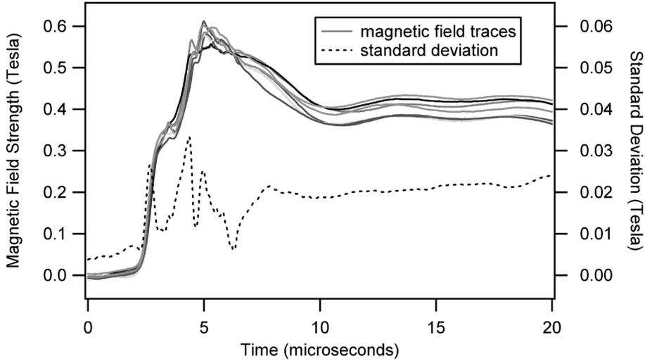
Figure 3: Magnetic field strength versus time for seven separate shots taken at the same physical location. The standard deviation of the seven measurements is also shown (dashed) on the right axis. The probe was located at position (12,4).
