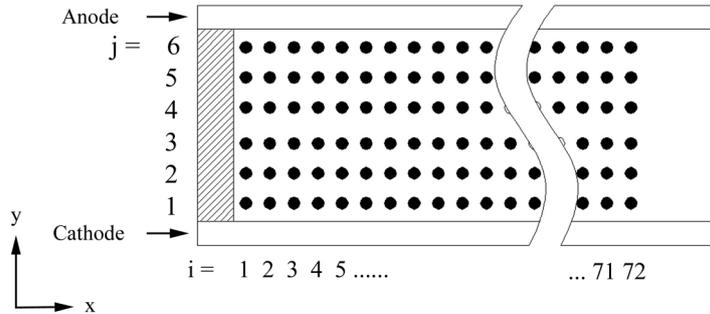
Figure 2: The array of measurement points in the accelerator is shown. The top copper plate is the anode, the bottom plate is the cathode. An insulator backplate is shown (shaded). The coordinate system is also defined. Note that the  $z$  direction is out of the page.
