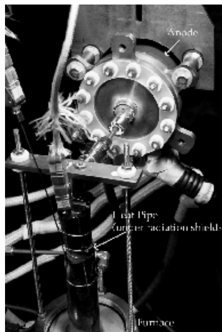
Figure 15: Close up back view showing heat pipe and thermocouples.
