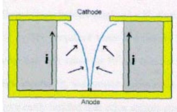
Figure 3: The magnetic forces of the AZPPT2 cause Teflon particles to be squeezed between the current sheets and directed out through the exhaust hole. Drawing from Levine [7]
