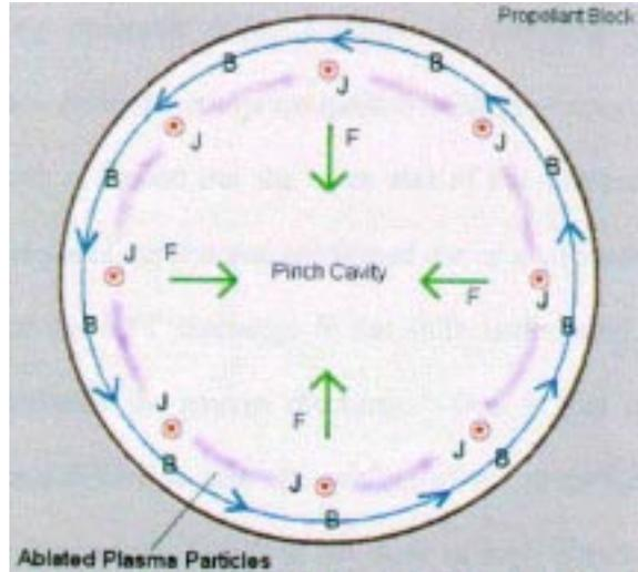
Figure 2: The ablated Teflon particles form a current conducting plasma inside the thruster. The current paths and corresponding magnetic fields are shown here in this figure from Levine [7].
