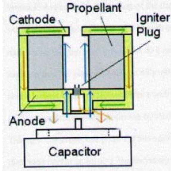
Figure 1: The geometry of the AZPPT2, as found in the work of Levine [7].
