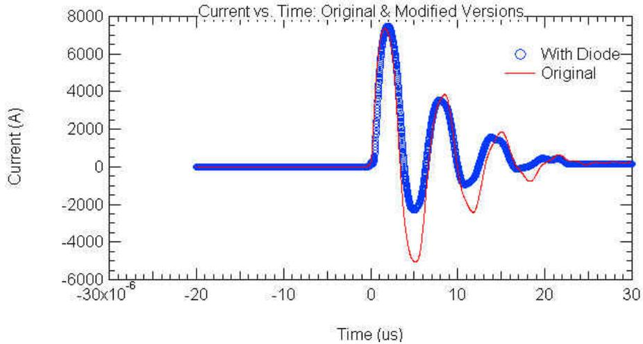
Figure 10: The current pattern from the new thruster is shown in comparison with a typical shot from the unmodified version.
