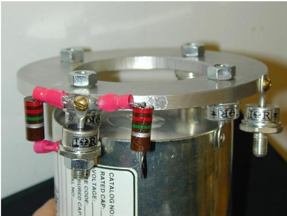
Figure 13: A photograph of the completed diode module.
