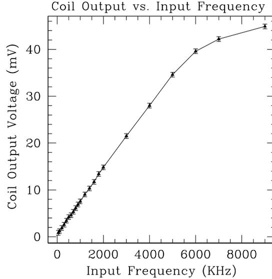
Figure 9: Output voltage of the Rogowski coil is shown as a function of input frequency for a sine wave current of constant peak-to-peak amplitude  $1.05 \pm 0.02$  A.
