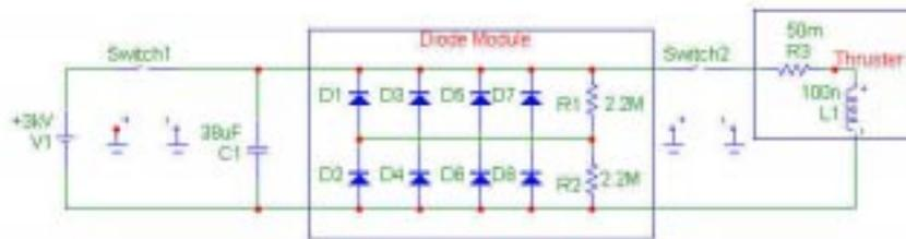
Figure 6: The diode module circuit; eight diodes are used because of the physical constraints of the available diodes.
