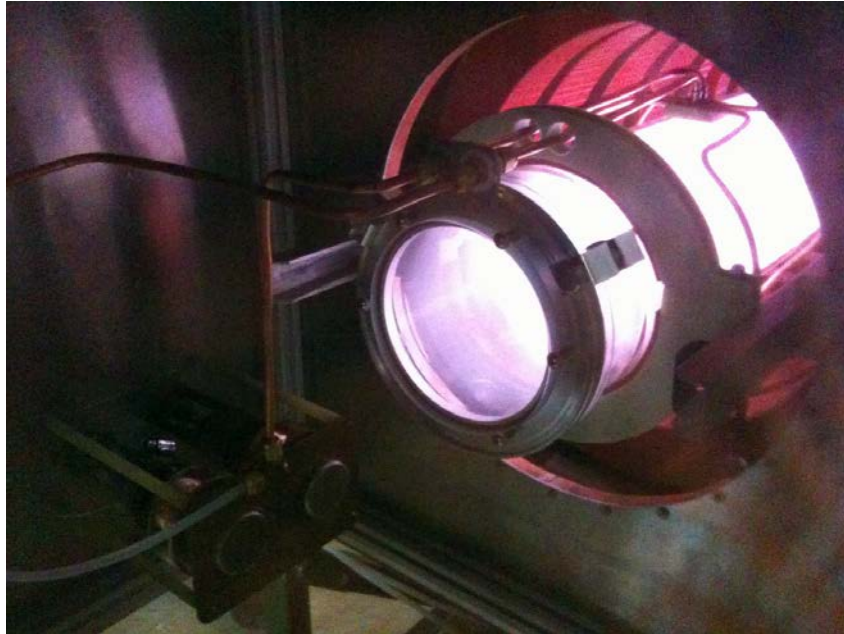
Figure 2. Photograph of one end of the experiment showing the plasma and part of the Boswell type saddle antenna wrapped around the vessel.
