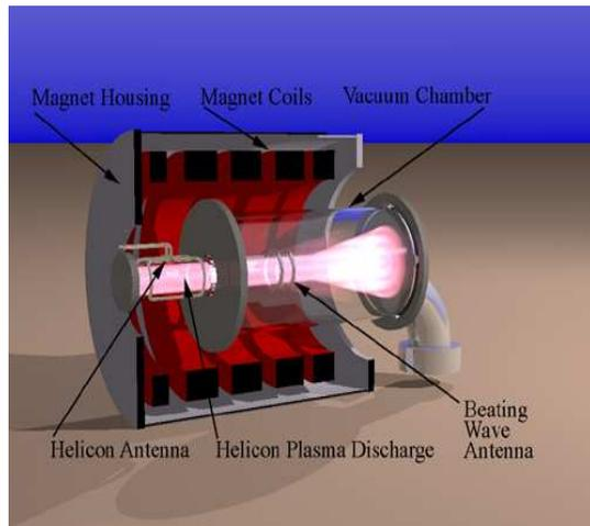
FIG. 3: Computer rendering of the experimental apparatus
