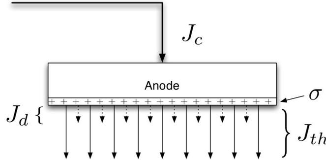
**Figure 3.** The anode as a current conduit, showing the current demanded by the power supply circuit ( $J_c$ ), the current supplied by the plasma ( $J_{th}$ ), and the displacement current ( $J_d$ ) representing the charging of the anode surface ( $\sigma$ ). Arrows not to scale;  $J_d \ll J_{th}$ .
