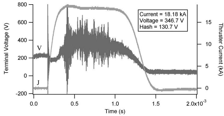
Figure 1. Typical voltage (V) and current (J) traces at an operating condition above onset for the Princeton FSBT,<sup>16</sup> operating with  $\dot{m} = 6$  g/s argon at 18 kA.
