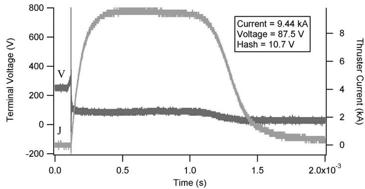
Figure 2. Typical voltage (V) and current (J) traces at an operating condition below onset for the Princeton FSBT,<sup>16</sup> operating with  $\dot{m} = 6$  g/s argon at 9 kA.
