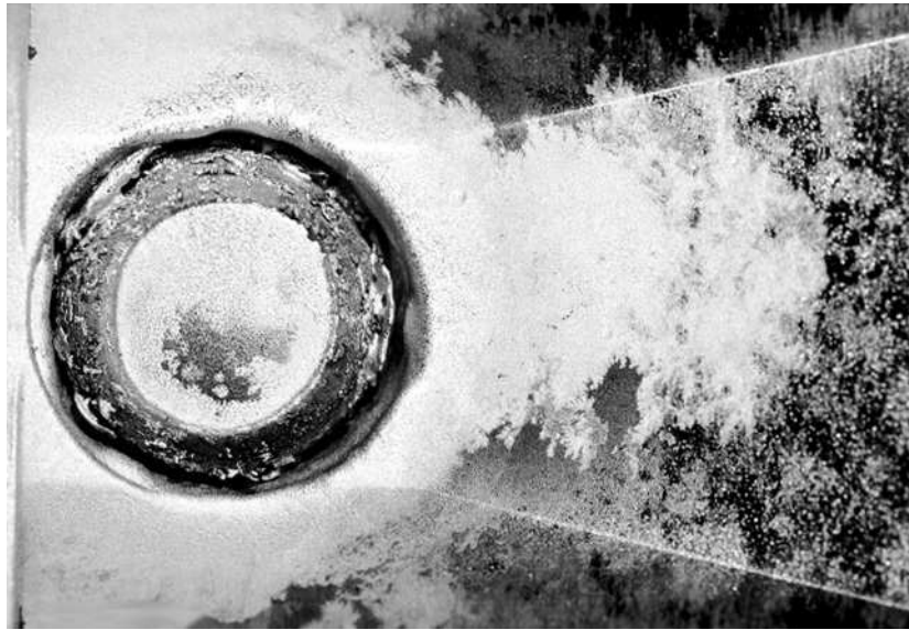
Figure 19: Cathode of SRL-EPPDyL PT7 showing the damage to the surface-flashover spark-plug after 1.5 million pulses.
